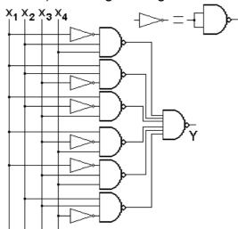
As for implementation in reality we rarely have access to multiple-input gates and most commonly used are 2-input gates, we have to be able to do it.
